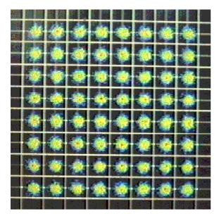
64 QAM signal with low broadband noise. Possible cause: Bad amplifier or to small of input level on an amplifier in the transmission line.
